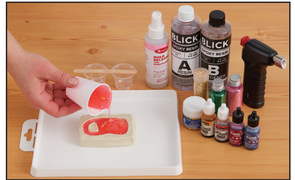
Step 2: Mix resin and hardener in a 1:1 ratio, add colorants as desired and pour into the mold.
