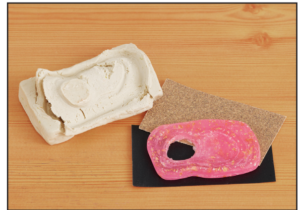
Step 3: Remove from the mold after 72 hours and buff rough edges with sandpaper.
